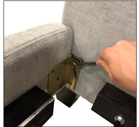
3. Tighten bolts to secure side rail
