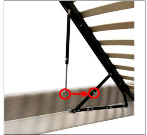
8. While someone holds the slats up, remove the mounting screw from the middle of the lift arm support. Place the end of the pneumatic lift over the post and replace the screw.
